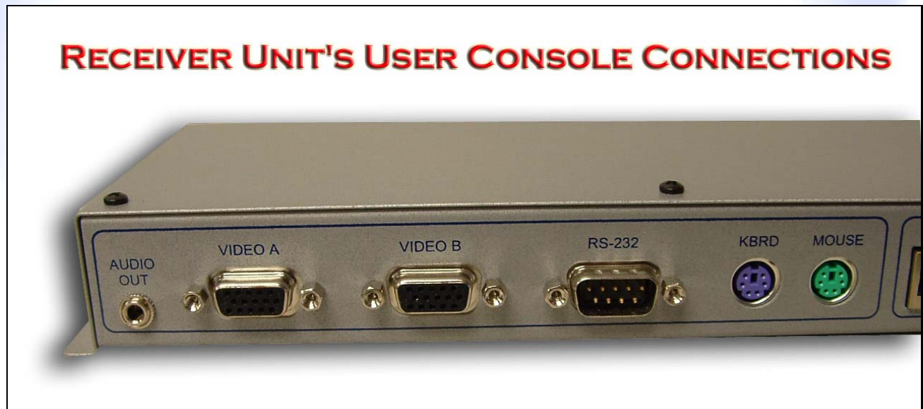
Figure 4 Receiver (Remote) Unit's Connections to User's Console
